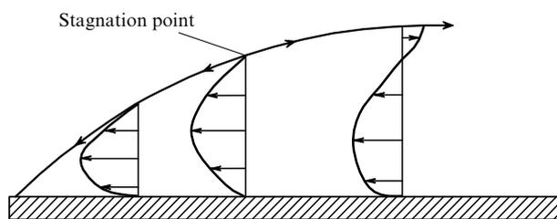
Figure 6. Emergence of a flow caused by the difference in surface tension coefficients.
