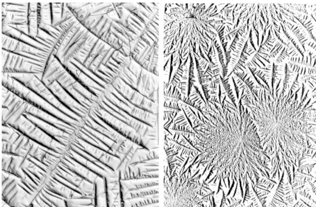
**Figure 8.** Dendrite in the samples of the aqueous solution of 0.9% NaCl and 8% albumin (at the left), and of 0.9% NaCl and 11% albumin (at the right). Both photographs were obtained at a similar magnification; the region measures about 1 mm.
