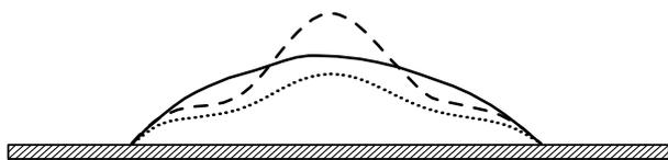
**Figure 7.** Schematic representation of the droplet profile dynamics on emergence of the buckling instability. The solid, dashed, and dotted lines depict the sequence of droplet profile variations.
