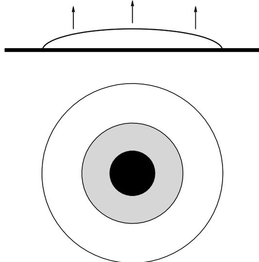
**Figure 1.** Schematic drawings of a droplet of biological fluid on a plane: the upper drawing shows the side elevation, and the lower one the top view. Shown in white is the region which primarily accumulates proteins when the droplet dries, in black the region which primarily accumulates salt, and in gray the transition region (taken from Ref. [2]).
