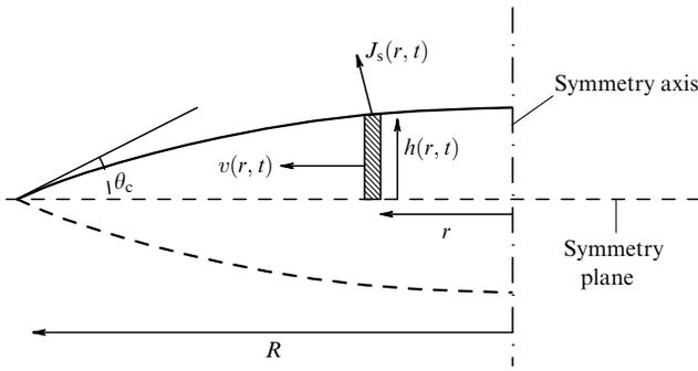
**Figure 5.** Schematic diagram illustrating the fluid mass conservation law [formula (1)].
